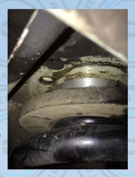
Please note that the above image was taken with a prototype spacer. Your spacers will be the same diameter as the upper spring isolator pad.
